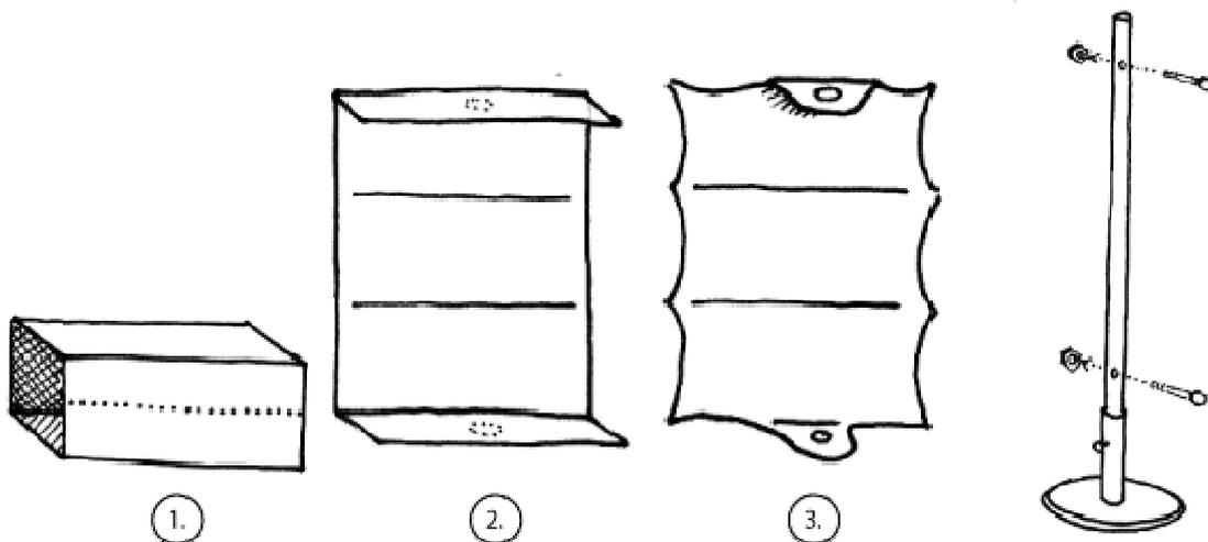
The mast is made from sticking an 8ft. (2" or 3" dia.) PVC pipe in a patio umbrella stand.
